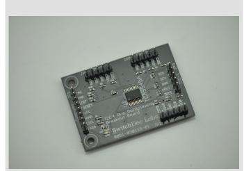
The **I2CMux Breakout Board** is an easy to use 4 Channel I2C Multiplexer.
