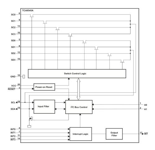
inputs (INT3'–INT0'), one for each of the downstream pairs, are provided. One interrupt (INT') output acts as an AND of the four interrupt inputs.
