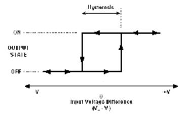
The diagram to the right shows a hysteresis 'loop' that describes how a comparator functions. The horizontal 'X' axis is the input, and represents the difference of the two input voltages. The vertical "Y" axis represents the comparator's output state.
