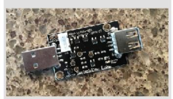
The **USB PowerControlV2** board is a USB to USB solid state relay.
