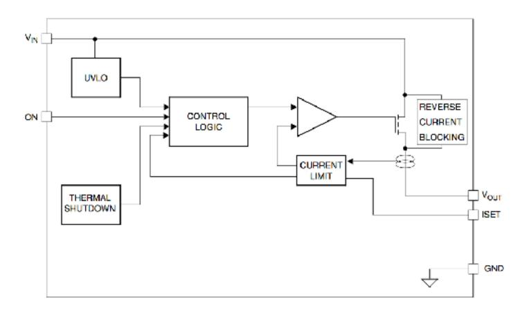
The FPF2123 provides full protection to systems and loads which may encounter large current conditions. These devices contain a 0.125 current-limited P-channel MOSFET which can operate over an input voltage range of 1.8-5.5V. The device is set for a minimum shutdown current of 1010mA with a maximum current shutdown of 1860mA. Internally, current is prevented from flowing when the MOSFET is off and the output
