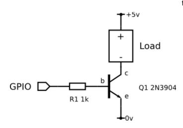
the LiPo Battery in your system or from a GPIO output pin on an Arduino. If you wish to control the USD PowerControl from a Raspberry Pi, you will need to use a level shifter as the logic high of the Raspberry Pi is only about 3.3V and will not turn on the board. You can do this also by using a single NPN transistor as shown below with a load resistor of about 10K Ohms.
