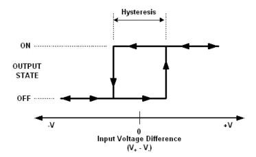
The diagram to the right shows a hysteresis 'loop' that describes how a comparator functions. The horizontal 'X' axis is the input, and represents the difference of the two input voltages. The vertical "Y" axis represents the comparator's output state.
