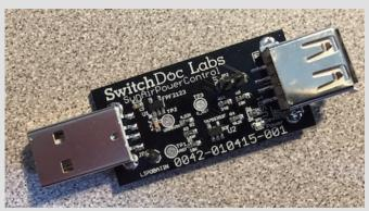
The **USB PowerControl** board is a USB to USB solid state relay.
