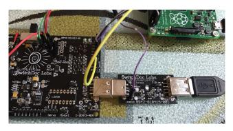
The USB PowerControl Board is a digitally controlled power switch for your Arduino or Raspberry Pi. Anything you can plug into a USB port can be controlled with USB PowerControl. It's easy to hook up. You connect a control line (a GPIO line or the output of a LiPo battery) to the LIPOBATIN line and if the line is LOW (< ~3.3V) the USB Port is off. If it is HIGH (above 3.8V) the USB Port is turned on and you have 5V of power to the USB plug.
