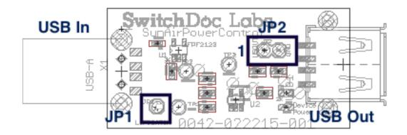
Physical dimensions of board: 65mm x 22.5mm x 12mm(max).
