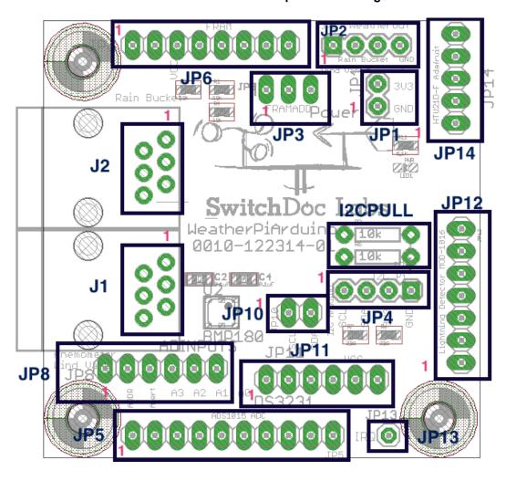
Physical dimensions of board: 50mm x 500mm x 14.5mm(max). Mounting holes inset 3.8mm x 3.8mm from each corner to center of hole. Diameter of hole 2mm.
