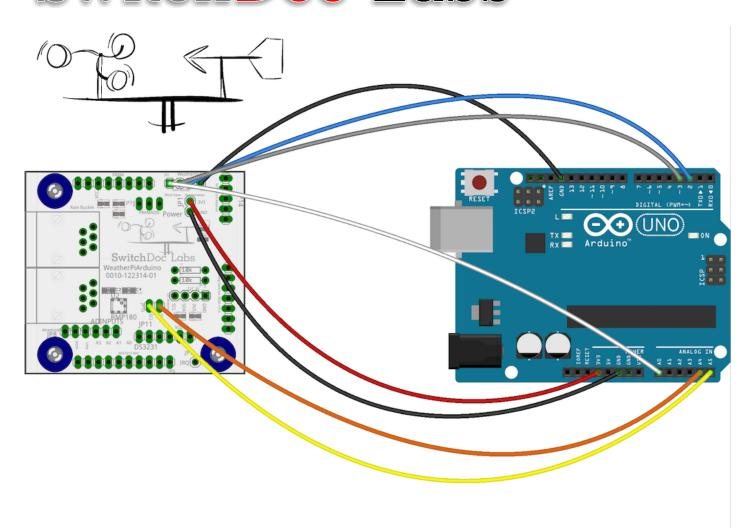
wind direction (as well as noise issues. If you have noise issues, bypass the Wind Vane line with 0.1uF bypass capacitors to ground.).
