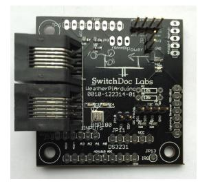
**WeatherPiArduino** is a weather station controller board designed to interface to Arduino and Raspberry Pi computers. It is an interface board developed by SwitchDoc Labs to allow the user to easily build a fully functioned Weather Station while allowing customization of functions.
