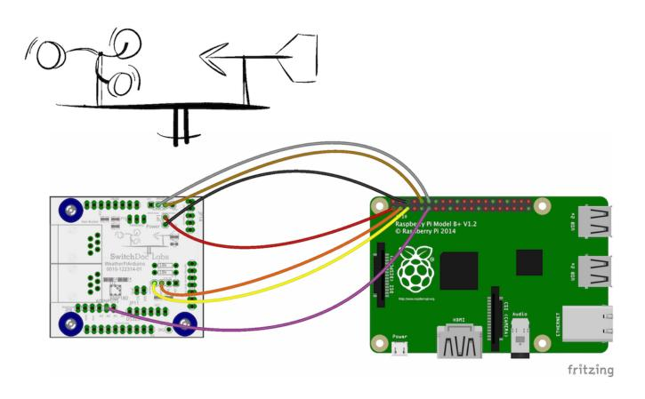
channels, or two differential channels. As a nice bonus, it even includes a programmable gain amplifier, up to x16, to help boost up smaller single/differential signals to the full range. This ADC can measure a large range of signals and its super easy to use. It is a great general purpose 12 bit converter.
