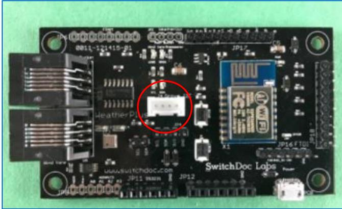
Version 1 with one Grove Connector. If this is the board you are working with, **skip to Step 9**.
