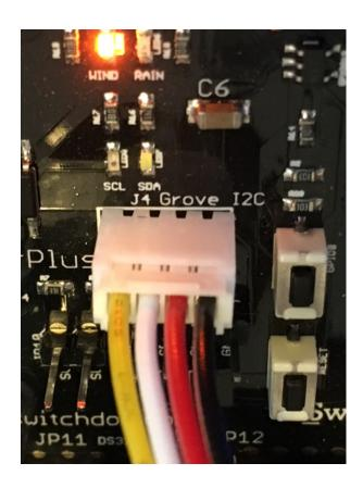
WeatherPlus boards before 0011-021916-01 only have one Grove connector, easily fixed with an inexpensive 4 channel Grove Hub.
