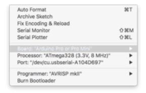
choose the 3.3V, 8MHz from the menu. This board runs at 8MHz to reduce current consumption.
