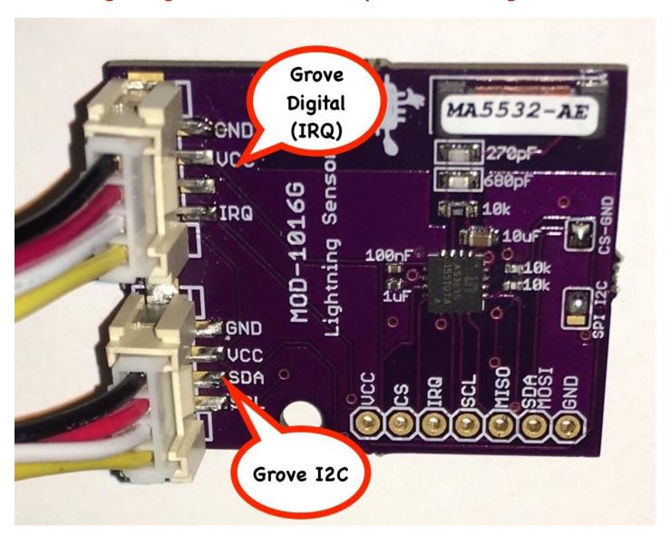
Physical dimensions of board: 35mm x 38mm x 10.0mm(max). Two mounting holes.
