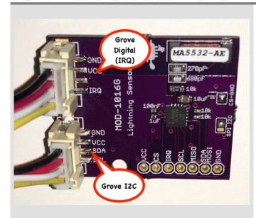
The **Grove Lightning Detector** is an Arduino and Raspberry Pi Grove compatible breakout board with a full set of connectors. No external antennas required! It is designed for use in Low Power applications such as battery and Solar Power applications. It can detect lighting up to 40km away.
