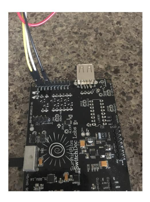
Step 3) Take the Multi Solar Panel Connector Board (Part C) and Plug in the F/F JST-PH2 (Part B) into the single connector (Labled TOCH and To SunAlrPlus) on the left side of the Multi Solar Panel Connector Board (Part C).
