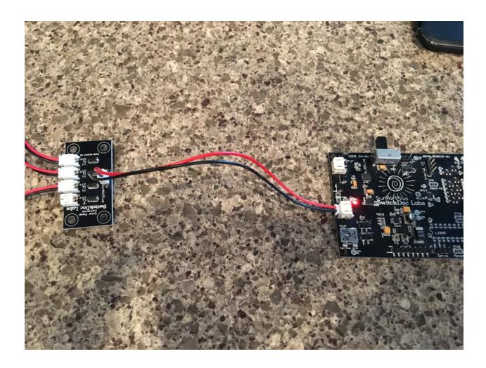
Step 6) Plug the Grove Cable (Part E) that you connected to SunAirPlus (Part D) in Step 2) into one of the Grove Connectors in OurWeather on the I2C Expansion Board. Check again to see that you did Step 2 correctly.
