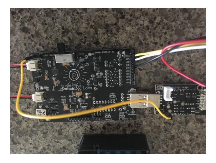
Step 10) Plug in your 3.7V LiPo (Lithium Poly) battery (NOT INCLUDED) into the BatteryJSTPH-2 Plug on SunAirPlus (Part D). Flip the SunAirPlus Power switch to the right as shown in the picture. If your LiPo battery is charged, the OurWeather should come on (the blue light will turn on on the USB PowerControl Board (Part F)). If it does not come on, then your LiPo battery is not charged enough to run OurWeather.
