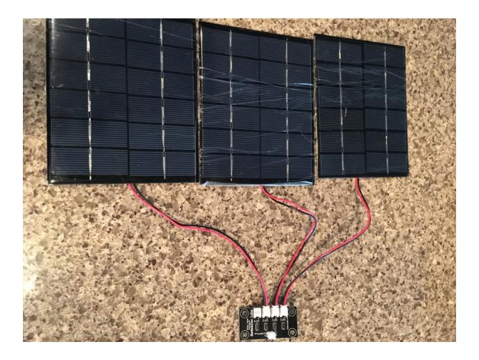
Step 5) Take end the F/F JSTPH-2 cable (Part B) not plugged into the Multi Solar Panel Connector Board (Part C) and plug it into the Solar Panel input on the SunAirPlus board (Part D). If you are in bright lights, you may see a red LED light up on the SunAirPlus board.
