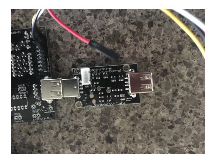
Step 8) Plug the USB Cable into the end of the USB PowerControl (Part F) and then into the MicroB plug on OurWeather. Note some wires are removed on the OurWeather station for clarity.
