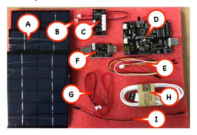
Part A - 3 (three) 330mA 6V Solar Panels (with JST-PH 2 Plugs soldered on back)
