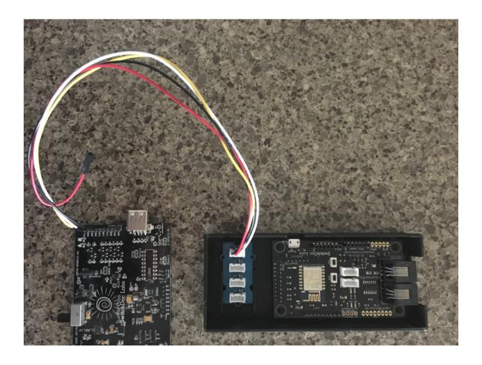
Step 7) Plug the USB PowerControl Board (Part F) into the USB A size Connector on SunAirPlus (Part D)
