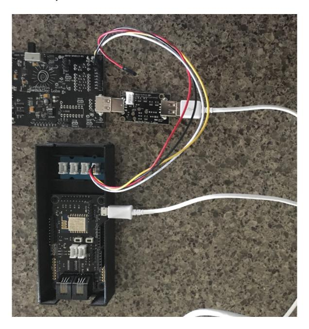
Step 9) Plug one end of the F/F Header Jumper wire (Part I) into the JP4 Single Pin header on SunAirPlus (Part D) and the other end into LIPOBATIN (JP5) on the USB PowerControl Board (Part F).
