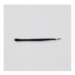
Simply remove the 10K surface mount resistor from the THERMISTOR pads (or cut the trace going to it), and solder in a 10K NTC thermistor in the provided holes. You can test out the temperature system by trying to charge while you place the thermistor in a freezer or against some ice, as well as in a cup of > 50°C hot water.
