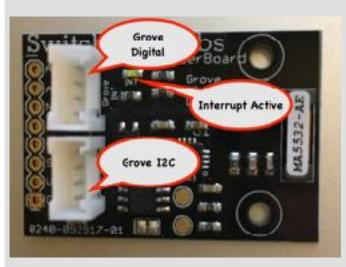
The **Thunder Board** is an Arduino and Raspberry Pi Grove compatible breakout board with a full set of connectors. No external antennas required! It is designed for use in Low Power applications such as battery and Solar Power applications. It can detect lighting up to 40km away. Features and Benefits:
