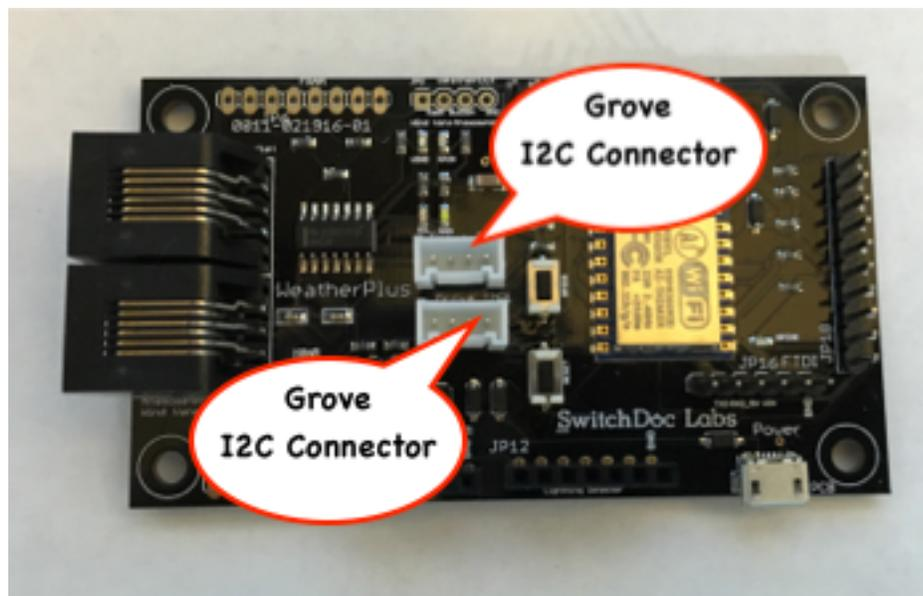
Step 2 - Plug the other end of the 20cm Grove Cable (Part C) into a 3.3V I2C Port (I2C is a bus so any of the top 3 will work) on Part B, the 3.3V to 5V I2C Converter and Hub. **NOTE:** We are using this board as an I2C Hub and using it to add additional pull-ups on the SDA and SCL lines on the I2C bus. Both sides of the board are actually wired to 3.3V on the WeatherPlus board.
