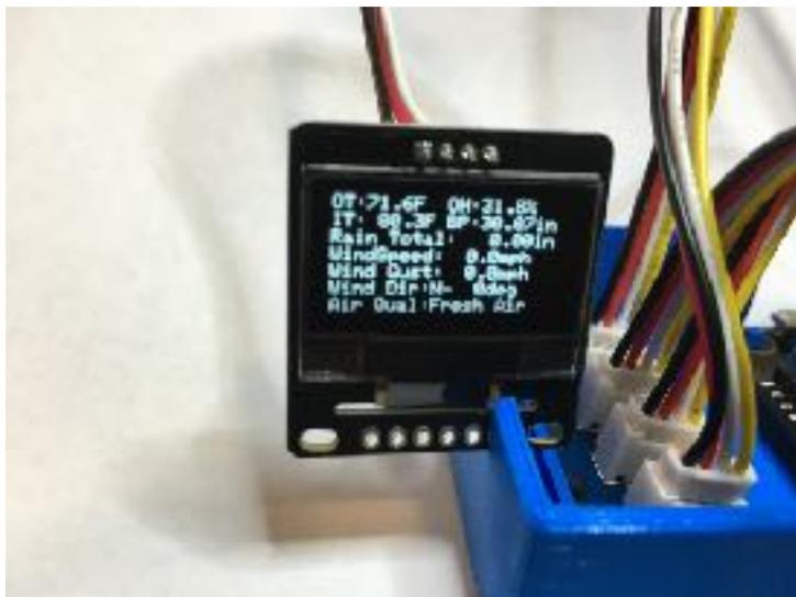
Step 2 - When the OLED display cycles around to show the weather information, you will see a lightning status screen by that will be blank, since there is no lightning reporting yet. You should see the light on the ThunderBoard turn on when you power the system and will turn off when OurWeather is running and checking the ThunderBoard for lightning.
