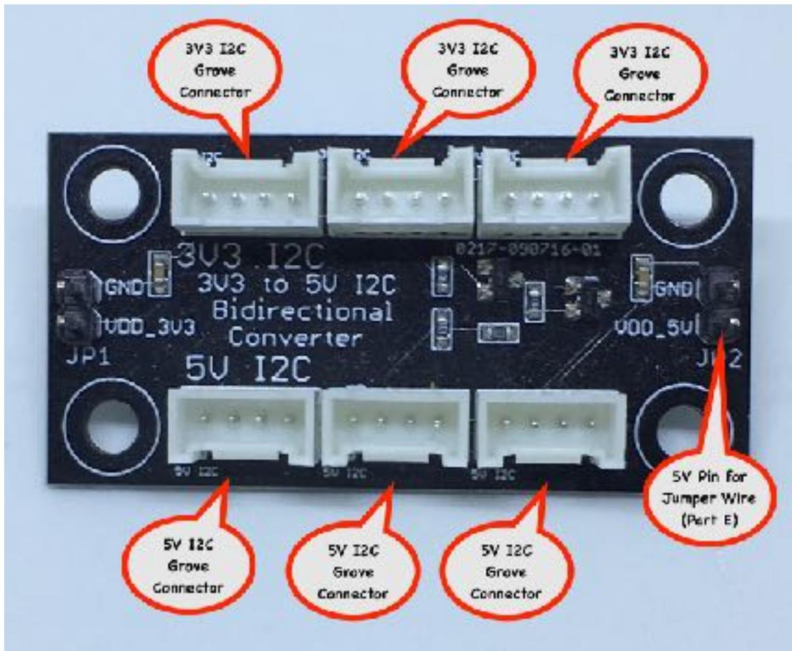
Step 3 - Plug the end of the 50cm Grove Cable (Part D) into one of the 5V I2C Grove Connectors on the 3.3V to 5V Converter Hub (Part B).
