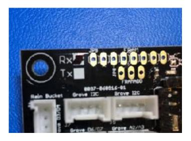
The two Mini Pro LP Boards are identical in hardware, but come preprogrammed with the TX (Transmitter) and RX (Receiver) software preprogrammed into the units. You can tell which is which by looking at the upper left corner of the Mini Pro LP Board. The black dot indicates that this board is an RX board. All the software is open source and you can change the software if you with.
