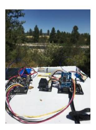
You can set the UART baud rate, frequency, output power, data rate, frequency deviation, receiving bandwidth parameters, etc. It comes pre-programmed for 433MHz and 9600 baud.
