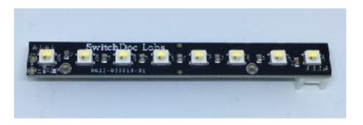
Physical dimensions of board: 101.5mm x 12.5mm x 10.0mm(max). Two mounting holes.
