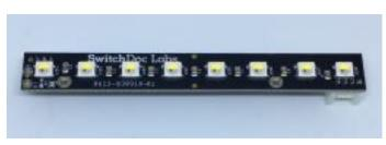
SwitchDoc Labs 8 Pixel Programmable RGBW Strip. This is a small chainable board with eight 5050 SK6812RGBW RGBW LEDs. The SK6812s are each individually addressable as the driver chip is located inside the LED. Each Stick has ~18mA constant current drive so the color will be very consistent even if the voltage varies, and requires near 5V.
