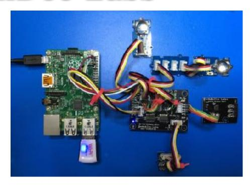
There are two types of Grove Connectors on the Grove Lightning Detector board, a Grove I2C connector and a Grove Digital connector for the Interrupt line to the microcontroller.
