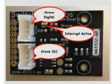
The **Thunder Board** is an Arduino and Raspberry Pi Grove compatible breakout board with a full set of connectors. No external antennas required! It is designed for use in Low Power applications such as battery and Solar Power applications. It can detect lighting up to 40km away.
