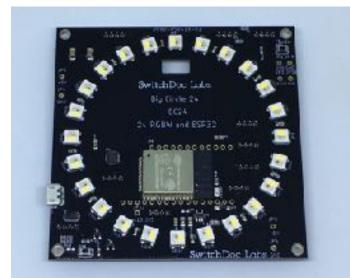
The BC24 is a novel use of programmable Pixel LEDs (RGBW programmable) in a perfect 24 segment circle combined with an powerful, highly connected on board computer (WiFi, Bluetooth, Bluetooth Low Power) called the ESP32.
