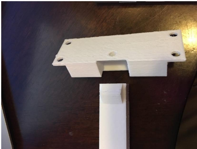
The complete bracket fits together as below. Secure with a screw into the Box.
