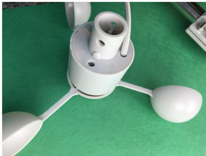
Step 16) Take a screw and bolt from **Part P-Screws for Mounting Weather Instruments to Brackets**, slide it into the **Part I-Wind Vane and Anemometer Bracket** under the **Part K-Anemometer** and tighten in place to secure the **Part K-Anemometer**.
