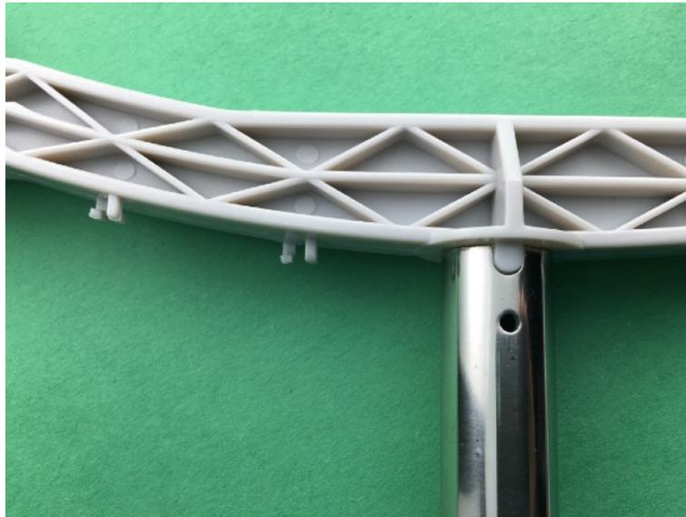
Step 13) Take a screw and bolt from **Part P-Screws for Mounting Weather Instruments to Brackets**, remove the bolt, slide the screw through the hole in the **Part N-Mounting Mast** from step and tighten the bolt to the Mast.
