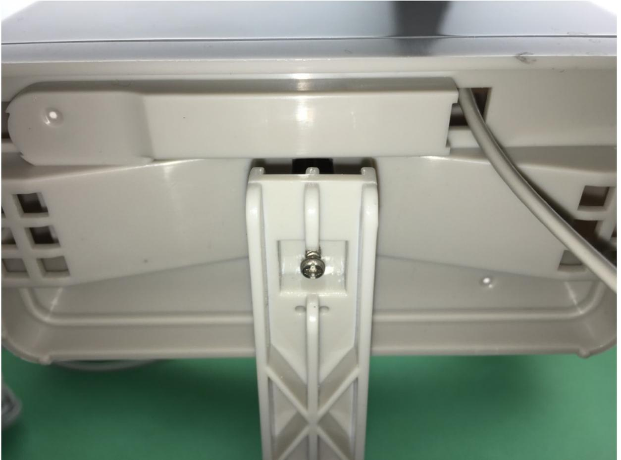
Step 22) - Push the second **Part N-Metal Mounting Mast for Weather Instruments** into the first **Part N-Metal Mounting Mast for Weather Instruments**.
