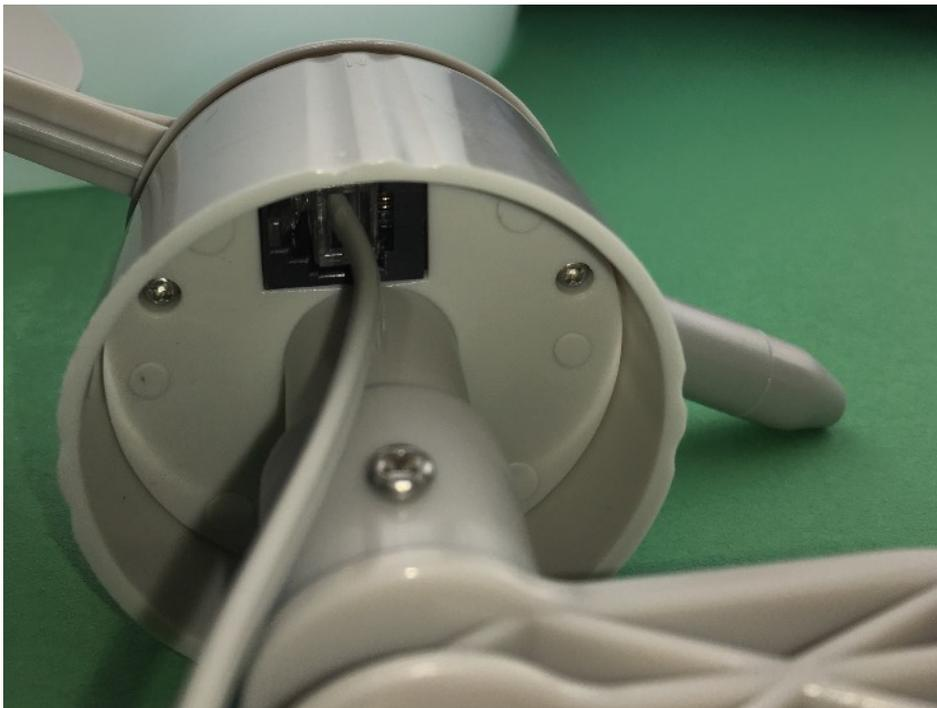
Step 20) Take the **Part J-Rain Gauge** and place it on the **Part L-Rain Gauge Mounting Assembly** perpendicular to the **Part L-Rain Gauge Mounting Assembly** as shown.
