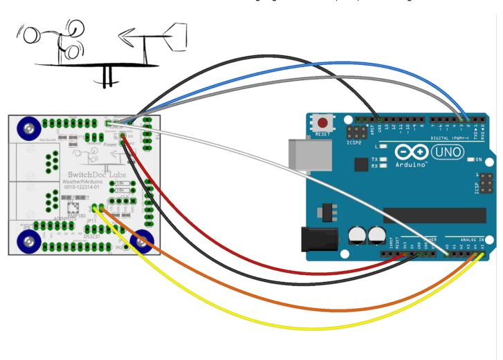
The Arduino contain an onboard 6 channel analog-to-digital (A/D) converter. The converter has 10 bit resolution, returning integers from 0 to 1024. The Arduino ADC does have some issues with accuracy and sample speed. If you have a long cable running to the WeatherRack sensors (Wind Vane especially), you will have issues reading the correct wind direction (as well as noise issues. If you have noise issues, bypass the Wind Vane line with 0.1uF bypass capacitors to ground.).
