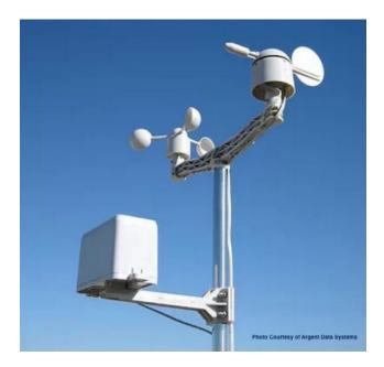
The SwitchDoc Labs WeatherRack Sensors provide a suite of weather sensors for use by Arduino and Raspberry Pi based small computers. It can also be used to connect with other computers and systems. It includes a Wind Vane, Anemometer and a tipping bucket Rain Gauge. Mounting hardware and a metal mast is also included. The included wires are terminated in RJ11 plugs. The WeatherRack is compatible with the SwitchDoc Labs WeatherPiArduino Weather Station Interface Board available on SwitchDoc.com.
