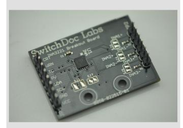
The **INA3221 Breakout Board** is an easy to use 3 Channel Current / Voltage I2C Monitor.
