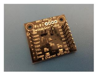
This board is an inexpensive I2C controlled 8 pin GPIO Extender Board (8GPIO).
