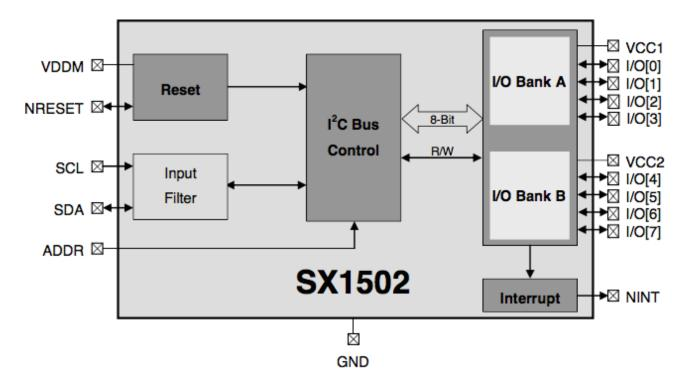
The SX1502 is a complete ultra low voltage General Purpose parallel Input/Output (GPIO) expanders ideal for low power handheld battery powered equipment. It allows easy serial expansion of I/O through a standard I2C interface. GPIO devices can provide additional control and monitoring when the microcontroller or
