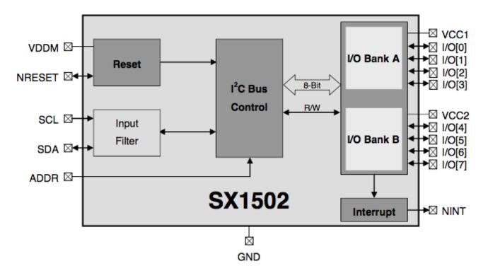
The SX1502 is a complete ultra low voltage General Purpose parallel Input/Output (GPIO) expanders ideal for low power handheld battery powered equipment. It allows easy serial expansion of I/O through a standard I2C interface. GPIO devices can provide additional control and monitoring when the microcontroller or chipset has insufficient I/O ports, or in systems where serial communication and control from a remote location is advantageous.
