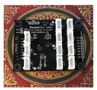
This board is an inexpensive Grove I2C controlled 8 pin GPIO Extender Board for the Raspberry Pi, Arduino and the ESP8266. It has 8 Grove Digital Connectors and 3 Grove I2C connectors (which form an I2C Hub).
