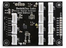
The **Grove Digital Extender board** is an easy to use I2C controlled board that provides 8 Grove Digital I/O ports.
