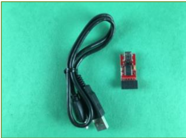
N – FTDI USB Cable for Computer to OurWeather Connection
