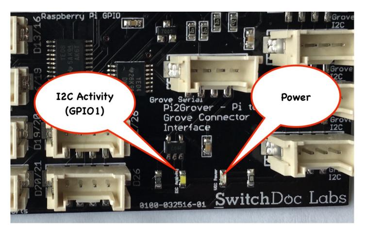
LED1 (Power) - On if Raspberry Pi is supplying 5V to the Pi2Grover Board
