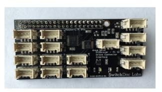
The Pi2Grover board provides 15 Grove connectors for your prototyping needs. 10 Grove Digital, 4 Grove I2C, and one Grove UART. Fast prototyping with many, many different Grove devices available. No software drivers required. You are right next to the hardware.
