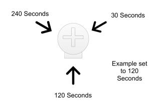
The timeout interval for each WatchDog timer is set by turning the respective TM1 / TM2 single turn potentiometer. It can be set from 30 seconds to 240 seconds. It is set by turning it over a 270 degree range.
