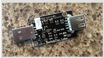
The **USB PowerControl** board is a USB to USB solid state relay. It comes in two flavors, one with an Active High Enable line and the other with an Active Low Enable line.
