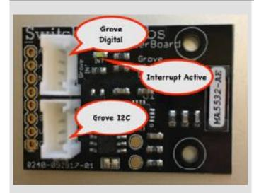
The **Thunder Board** is an Arduino and Raspberry Pi Grove compatible breakout board with a full set of connectors. No external antennas required! It is designed for use in Low Power applications such as battery and Solar Power applications. It can detect lighting up to 40km away.
