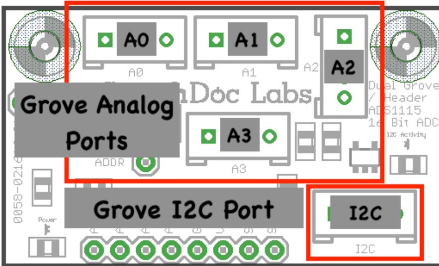
**Step 11)** Connect the 20cm cable (Part M) plugged into the OLED Display (Part E) into the I2C Plug (any I2C Plug – it’s a bus) on the Pi2Grover (Part A)
