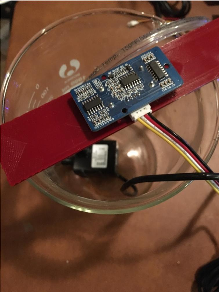
Step 3) In the SDL\_Pi\_SmartGardenSystem directory run the following CalibrateWaterTank program and following the on screen directions. Do NOT get the Ultrasonic Sensor wet and don't fill the tank so full that the sensors will be in the water! This program writes a calibration file containing these full and empty measurement numbers. If you change the tank size or depth, just re-run this calibration program.
