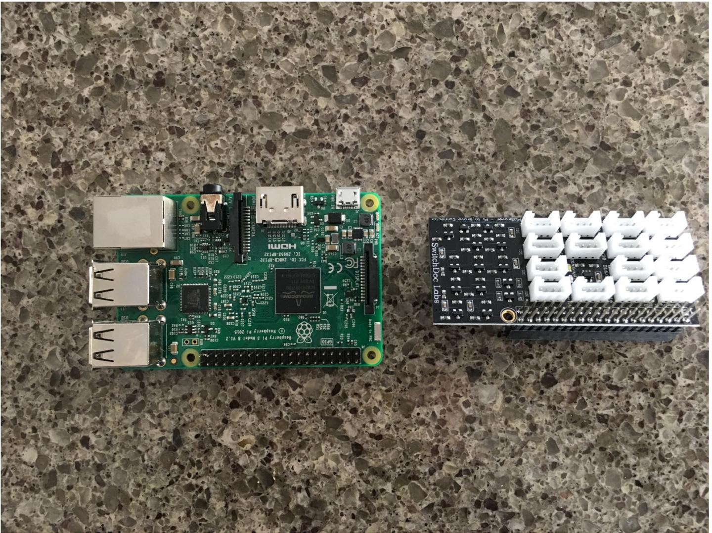
**Step 7)** Making sure you align the pins correctly gently press the Pi2Grover Board (Part A) onto the 40 pin GPIO connector on the Raspberry Pi
