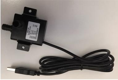
**Step 19)** Take the USB Submersible Pump (Part K) and plug the USB cord into the USB Port on the USB PowerControlNE (Part P). Then take a 20cm Grove Cable (Part M) and plug it into the Grove Connector on the USB PowerControlNE (Part P) and the other end into the Pi2Grover (Part A) in the D16/D19 Connector.
