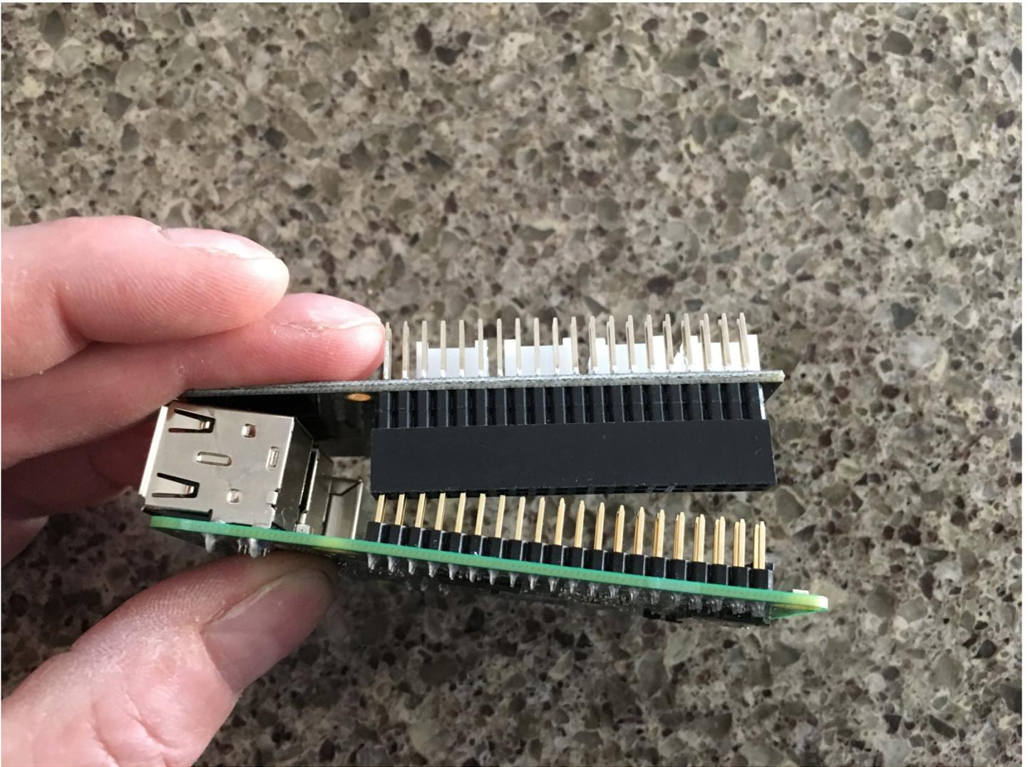
**Step 8)** Gently finish pushing the Pi2Grover (Part A) onto the Raspberry Pi GPIO pins, making sure the pins are aligned. There will be no pins showing on either end.
