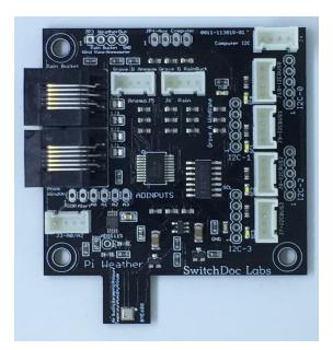
Raspberry Pi computers. It is an interface board developed by SwitchDoc Labs to allow the user to easily build a fully functioned Weather Station while allowing customization of functions.
