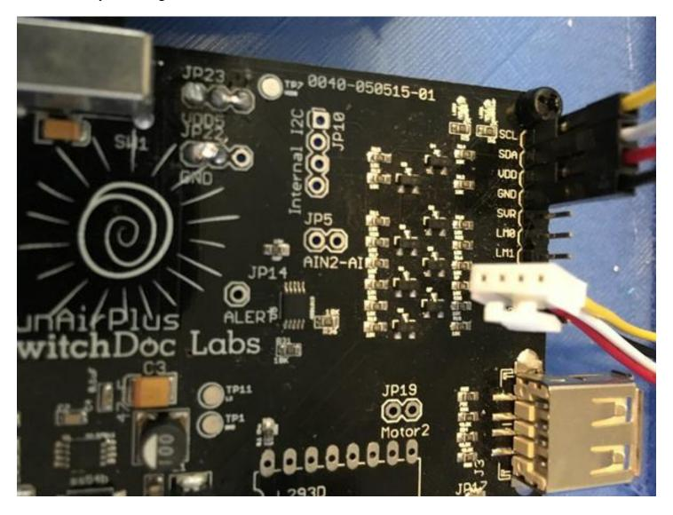
**Step 6**) Plug the Grove Cable from SunAirPlus (Part AD) to one of the I2C Ports on the Mini Pro LP Board (Part AB).
