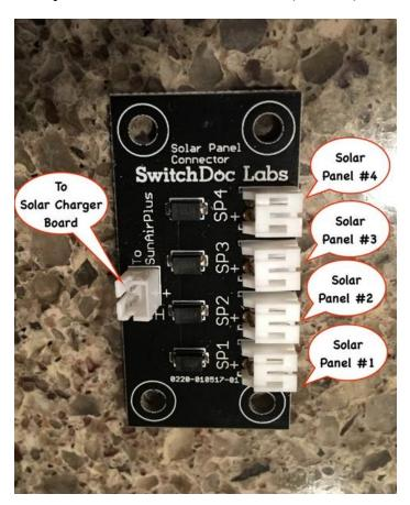
**Step 14)** Plug the JST2 Plug on the other 330mA Solar Panels (Part AE) into the Solar Panel #2 Plug on the Multiple Solar Panel Connector Board (Part AH).
