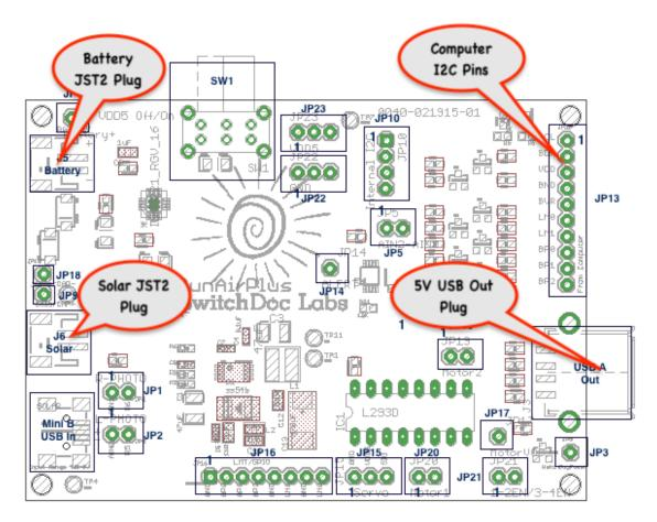
**Step 16**) Plus the USB Type A to Micro USB Cable (Part AG) from the 5V USB Out Plug on SunAirPlus (Part AD) to the MicroUSB Plug on the Mini Pro LP (Part AB).
