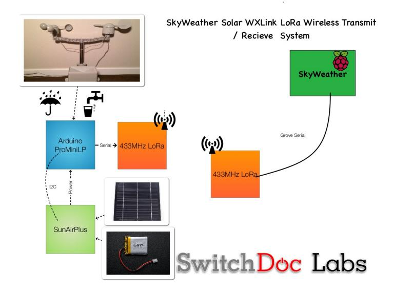
The issue is sometimes you don't want to run a wire all the way from the Weather Station to the wind and rain sensor. Using the Mini Pro LP, we built a WeatherRack reader and then we use a transmitter to send it back to the SkyWeather station inside. We then added solar power to the system.
