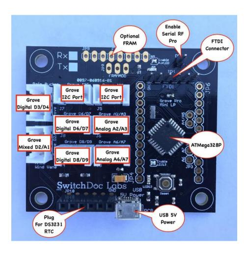
**Step 7**) Plug the Grove Cable from the AM2315 Temperature / Humidity Sensor (that you disconnected from SkyWeather in Step 2) into the other I2C Port on the Mini Pro LP Board (Part AB).
