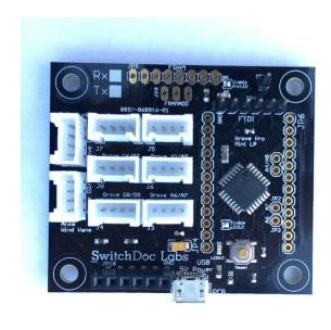
Part AC – WXLinkWR – WeatherRack Interface Board
