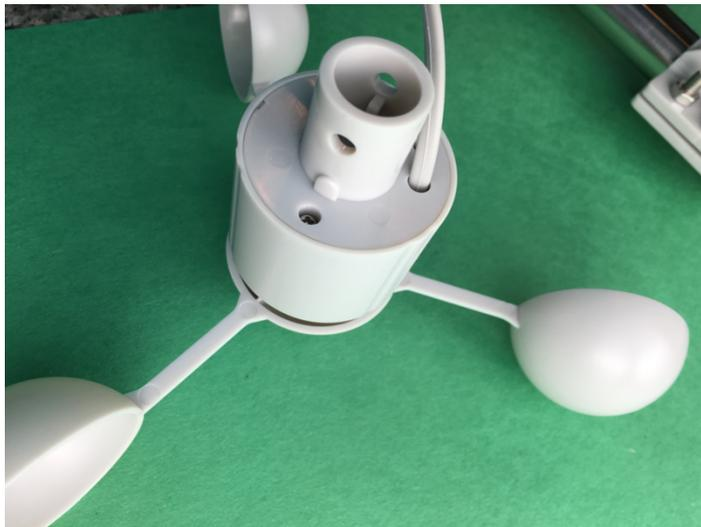
**Step 27)** Take a screw and nut (Part P), slide it into the Wind Vane and Anemometer Bracket (Part H) under the Anemometer (Part J) and tighten in place to secure the Anemometer (Part J).
