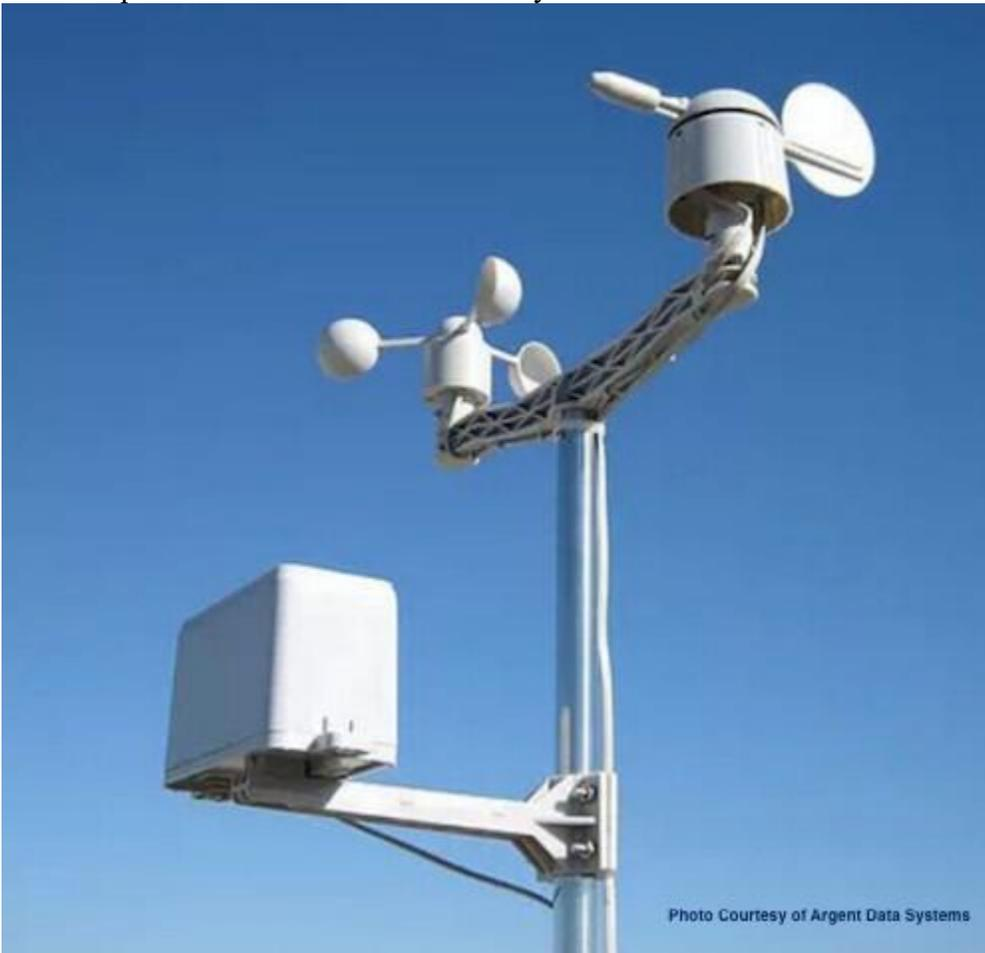
Note that you have clamps and wire ties left over in the assembly process for the WeatherRack. You can use these to install the WeatherRack assembly outdoors and use the wire ties to secure the cables from the WeatherRack.
