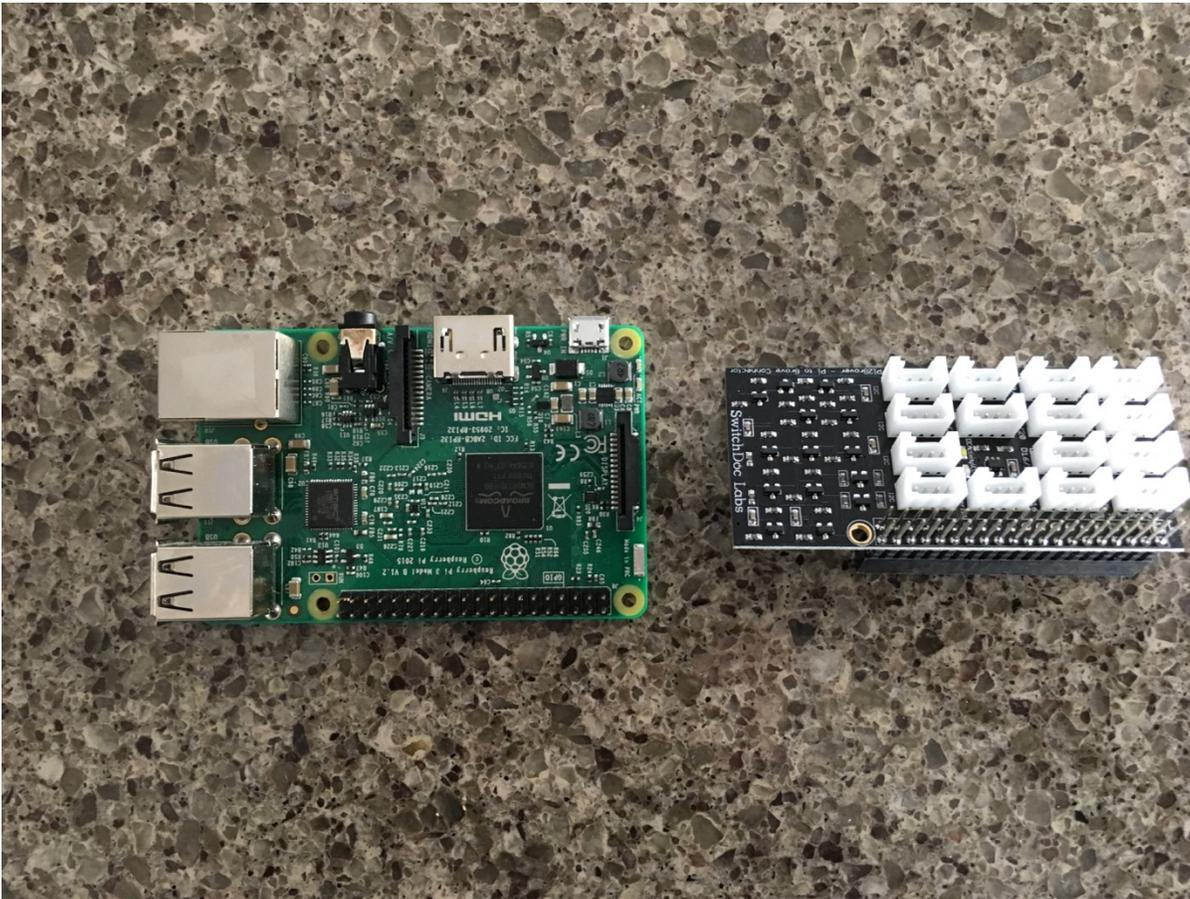
**Step 4)** Making sure you align the pins correctly gently press the Pi2Grover Board (Part A) onto the 40 pin GPIO connector on the Raspberry Pi
