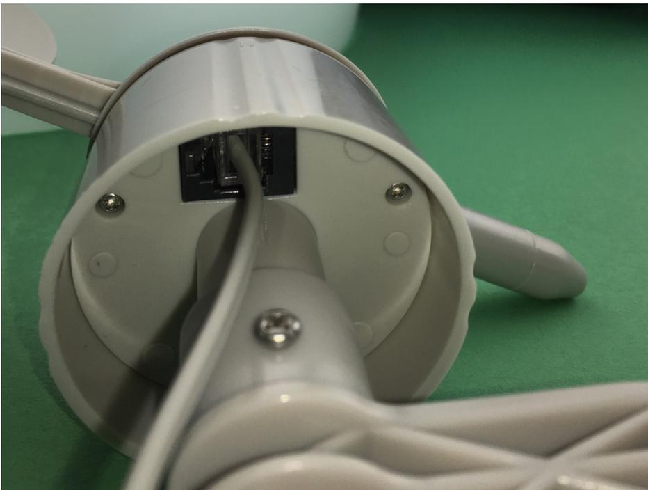
**Step 31)** Take the Rain Gauge (Part I) and place it on the Rain Gauge Mounting Assembly (Part K)
