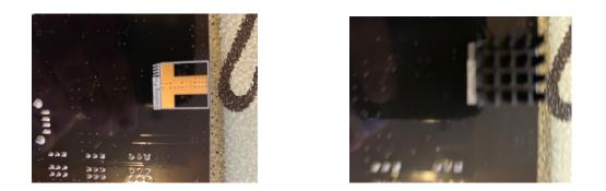
Step 5) Set the DIP Switch on the Solar Charger(Part D) to 12V MPPT for the most efficient charging.
