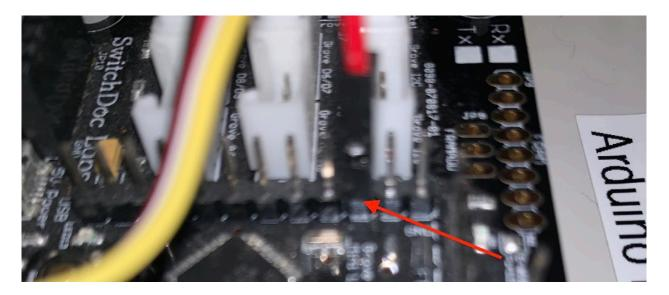
Page 20 Version 1.1 August 2019 If your jumper wires are loose, then put a drop of super glue at the place where the jumper meets the header. This will secure them.
