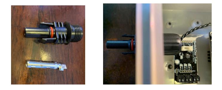
Step 2) Place the other end of the black wire into the "-" terminal of the Solar Charger SOLAR IN terminal.
