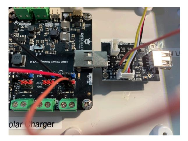
Step 2) Take a Female to Female single wire jumpier and connect it to the Arduino Reset on plug JP4 on the WatchDog Timer board (see picture).
