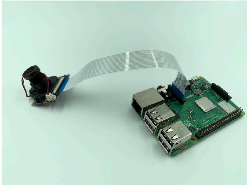
**Step 3)** Using 4 M2 Screws (Part P), screw your Raspberry Pi (Part A) into the MouseAir Base (Part M) oriented as shown. Mount your Pi Camera (Part D) using the top holes of the stand and the Pi Camera using two M2 Screws and nuts.
