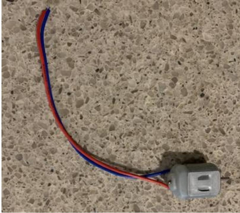
**Part J - Launch Motor #2      1101-5VDCMOTOR-DSBT (same as Part I)**
