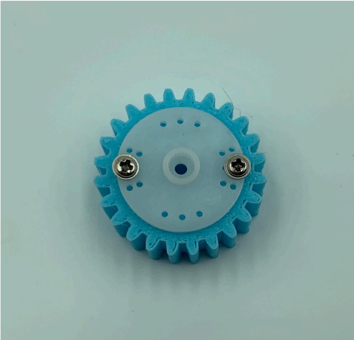
**Step 5)** Push the Gear on the FS90R Servo Motor (Part K) and gently snap the assembly as shown into the MouseAir Base Plate (Part M).
