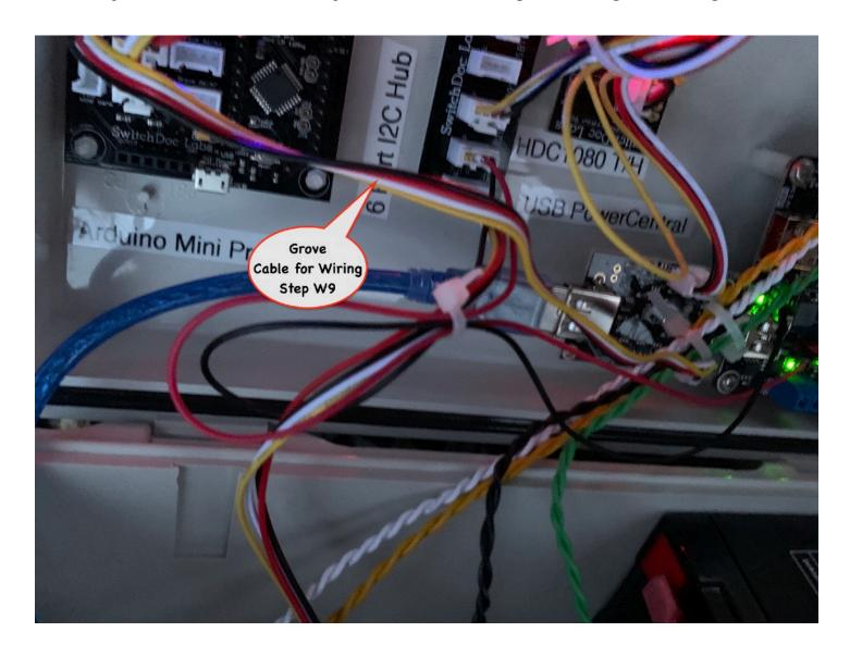
This completes the Grove Wiring for SolarMAX LiPo. Next is the jumper wiring.
