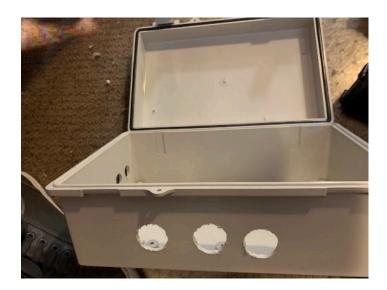
**Step 3)** Insert Part F - USB Weatherproof Plug into the BUD Box, with the cap on the outside in the rightmost 1" hole. Screw down.
