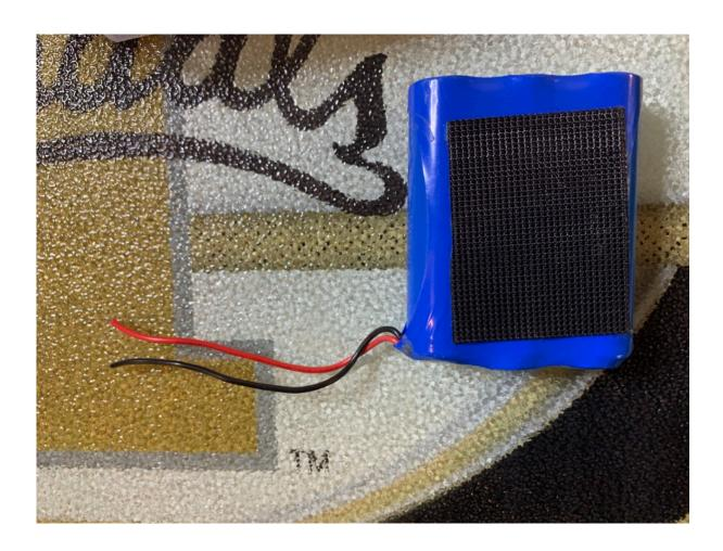
**Step 4) WARNING SOLDERING STEP -** Solder the plus (likely red) wire on the battery to the 26cm Red wire on the cable you built in Step 2). Insulate this connection with electrical tape.
