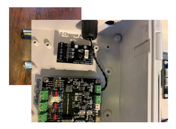
Step 2) Place the other end of the black wire into the "-" terminal of the Solar Charger SOLAR IN terminal.
