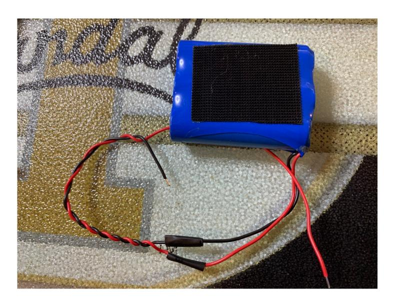
**Step 6) FINAL BATTERY INSTALLATION! BE CAREFUL.** Don't short the wires or touch them to other hardware in the box. Take your battery assembly and velcro or otherwise secure it to the box. Take the black wire (Ground) and connect it to the "-" screw terminal on 3.7V BAT IN on the Solar Charger board (Part D)
