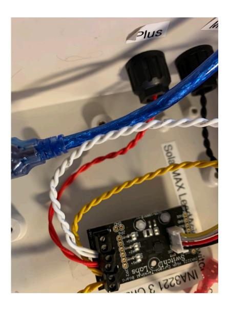
**Step 4)** Using Red 38cm long wires (We used White in the pictures above), braid them together and strip the ends. Run this wire from the 3 Channel INA3221 ADC (Part C) IN2- screw terminal to the "+ terminal on the Solar Charger (Part D) in the SOLAR IN block.
