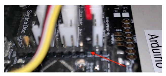
If your jumper wires are loose, then put a drop of super glue at the place where the jumper meets the header. This will secure them.
