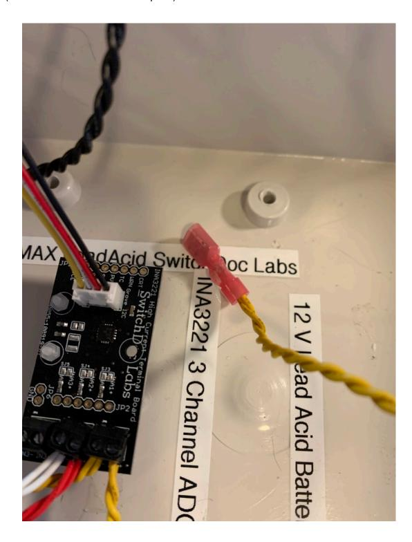
**Step 4)** Take the Yellow Cold Press Crimp spade connector and place the Green Wires (From the 12V BATIN "-" Screw Connector on the Solar Controller Board (Part D) into the spade connector and crimp the connector to hold the wires in place (and make connection with the spade).
