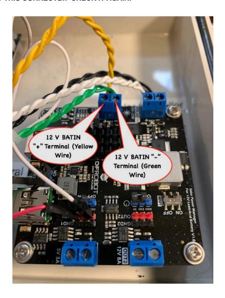
**Step 2)** Cut two 26cm Green wires, braid them and strip both ends. Connect on end of the Green wires to the 12V BATIN "-" screw terminal as shown in the picture above.
