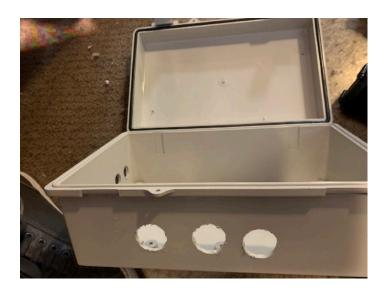
**Step 3)** Insert Part F - USB Weatherproof Plug into the BUD Box, with the cap on the outside in the rightmost 1" hole. Screw down.
