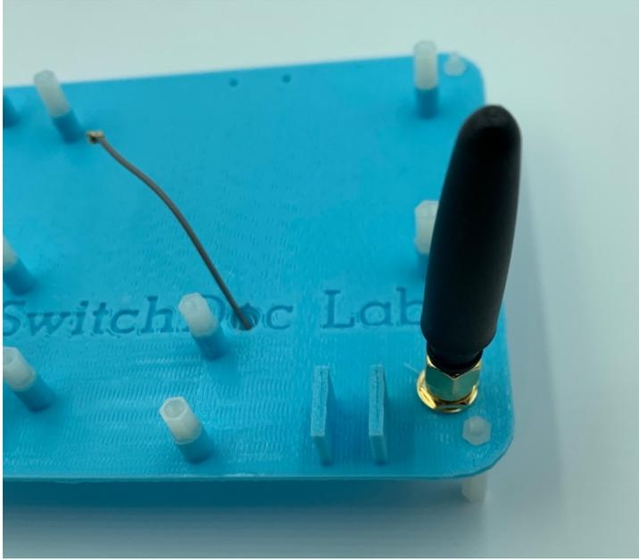
Step 5 – Attach the WeatherPlus2 Board (R) to the OurWeather Base unit (Q) using four screws from the M2 Nylon box (E). Take the small gold part of the WiFi Antenna Wire (C) and push it gently down on the
