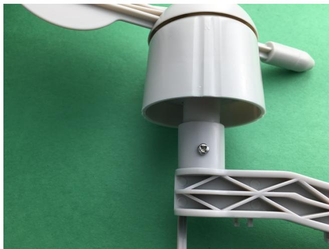
under the Wind Vane (G) and tighten in place to secure the Wind Vane.
