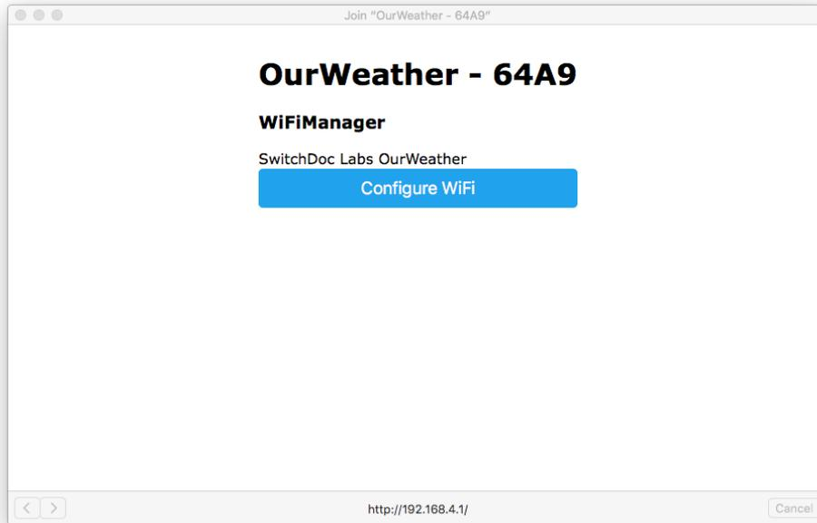
versions) and type in “<http://192.168.4.1>” and shortly you will see a screen as below. Note that you only have 5 minutes to complete the next steps. Otherwise OurWeather will start displaying the weather data. If you wish to restart, either repeat Steps 1-3 or push the reset button on the Weather Plus board.
