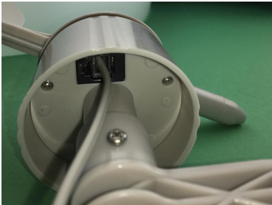
Step 18 - Take the Rain Gauge (I) and place it on the Rain Gauge Mounting Assembly (K)
