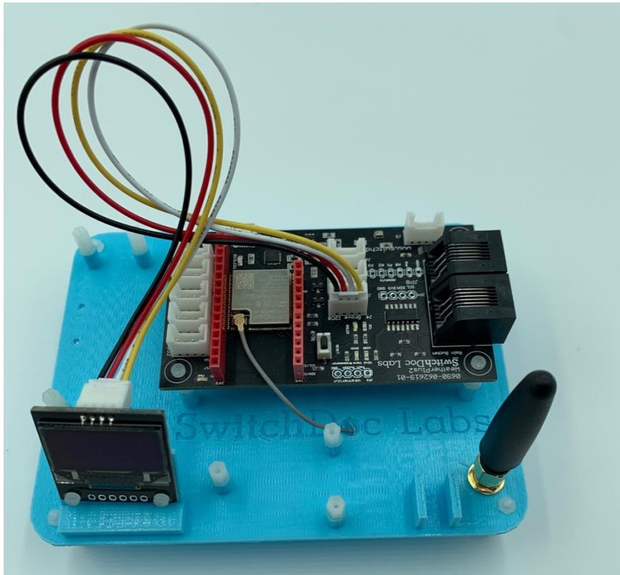
Step 7 - Plug in the Grove connector from the SHT30 Outdoor Temp/Humidity Sensor (D) into the I2C Grove Connector Slot on the WeatherPlus2 (Q) Any I2C Grove socket will work, use the one on the back of the WeatherPlus2 Board(Q).
