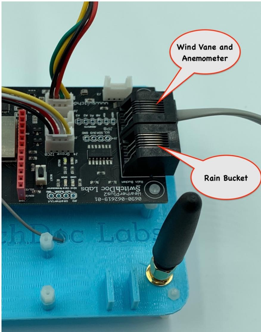
Step 23 - Plug the RJ54 Cable coming from the Rain Bucket (I) into the RJ54 Plug receptacle on the WeatherPlus board (R). One is labeled Rain Bucket and the other is labeled Anemometer/Wind Vane. If you plug them in the wrong position, nothing will be damaged, but the Weather sensors will not work until you plug them in correctly.
