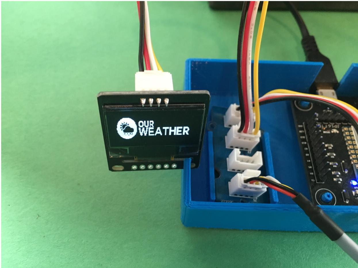
Step 3 - Wait 10 minutes and then you will see the OurWeather OLED Display (B) start to cycle through current weather conditions.
