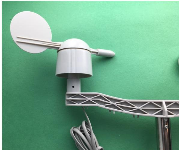
Anemometer Bracket (H). Note the alignment tab on the Wind Vane.
