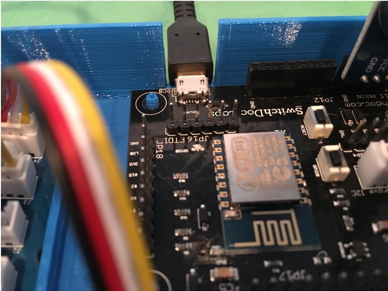
Step 2 - Plug in the Wall unit of the 5V Power Supply (A) into a 110V AC outlet. You will then see the OurWeather Logo on the OLED Display (B). If you don;t see the Logo then see the Troubleshooting section at the end of this manual.
