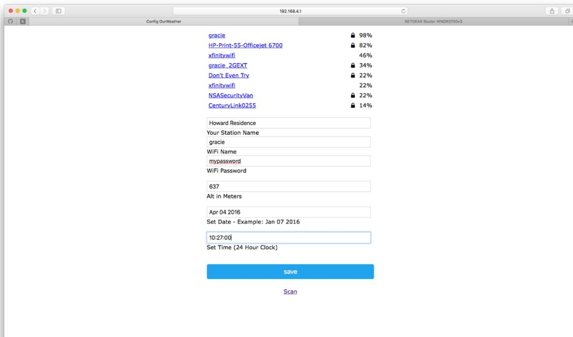
Step 9: Hit Save. OurWeather will try to connect. If it doesn't connect (for example if you typed a bad password or WiFi name - watch the screen) then it will reset it self back to Step 4 and you can try again.
