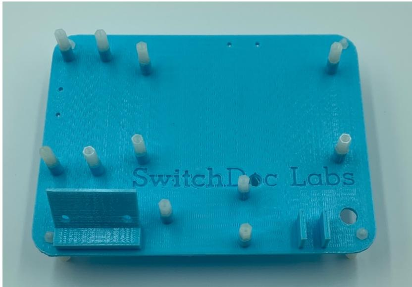
Step 2 – Using Super Glue, place a standoff (E) in each of the remain pylon holes on the OurWeather Base 3D Print (Q). Let dry.
