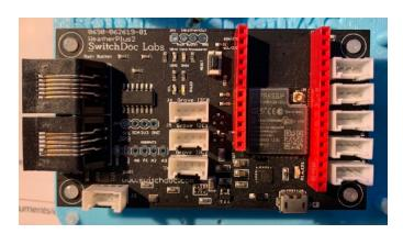
WeatherPlus2 is a complete weather station controller board designed to interface to Arduino and Raspberry Pi computers. It contains a full Arduino Compatible ESP32 Wifi computer and can run stand-alone or with a Raspberry Pi or Arduino
