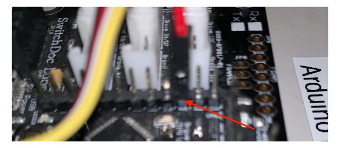
Page 22 Version 1.5 March 2020 If your jumper wires are loose, then put a drop of super glue at the place where the jumper meets the header. This will secure them.
