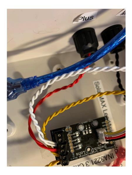
Page 15 Version 1.5 March 2020 **Step 4)** Using Red 38cm long wires (We used White in the pictures above), braid them together and strip the ends. Run this wire from the 3 Channel INA3221 ADC (Part C) IN2- screw terminal to the "+ terminal on the Solar Charger (Part D) in the SOLAR IN block.
