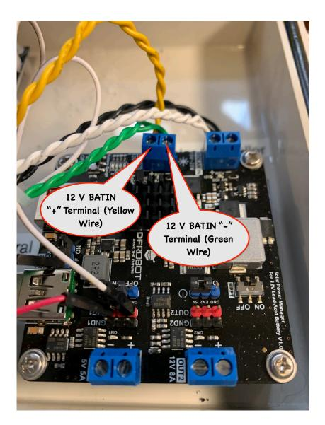
**Step 2)** Cut two 26cm Green wires, braid them and strip both ends. Connect on end of the Green wires to the 12V BATIN "-" screw terminal as shown in the picture above.
