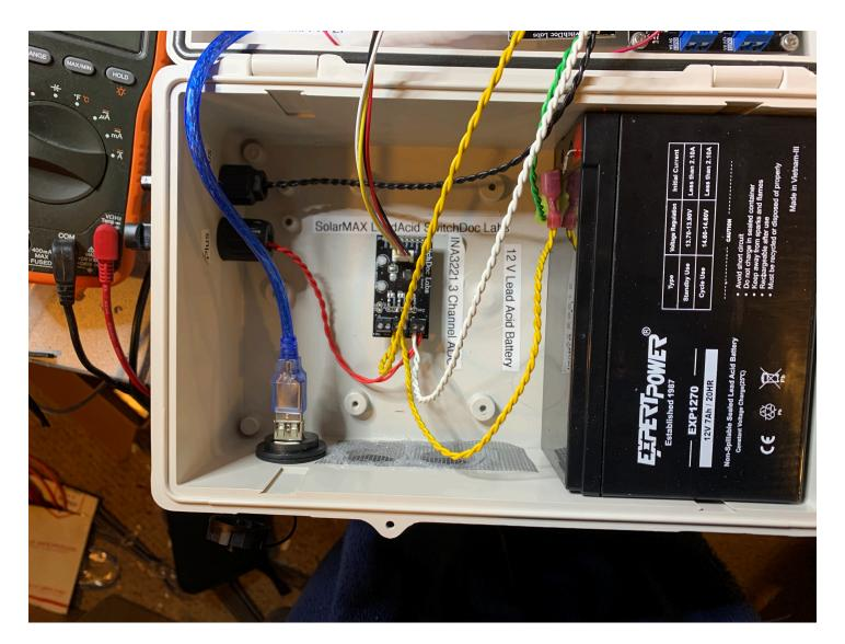
**Step 2)** Slide the Yellow Spade connector (connected to the Green wire which is connected to the "-" terminal on the Solar Control (Part D) 12V BATIN "-" screw down terminal) on the **Negative** Spade on the 12 V Battery (CHECK YOUR WORK!!!!)
