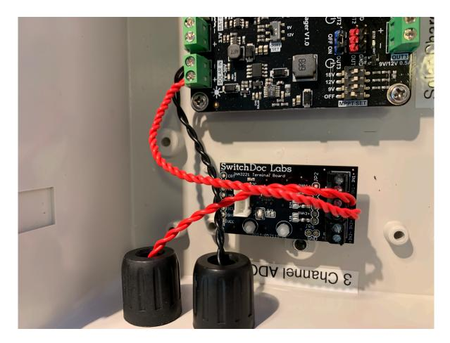
**Step 3**) Using red 14cm long wires, braid them together, strip, crimp then and assemble the female MC4 and install it in the Plus Hole in the box. Run the end of this wire to the 3 Channel ADC (Part C) and secure them in the IN2+ screw terminal.
