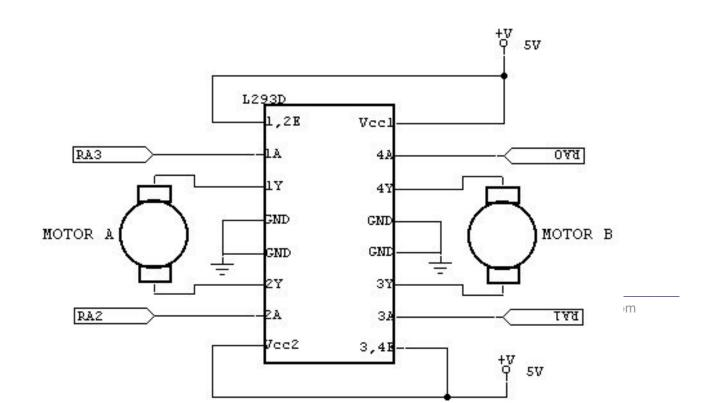
Figure 6: Block Diagram of L293D Connected to a Stepper Motor
