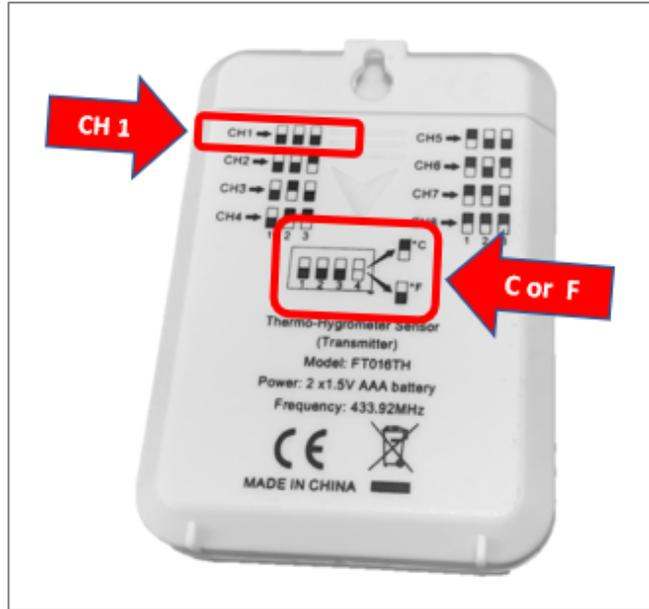
**Step 2:** Put two AA batteries in the battery compartment of the Indoor Wireless Sensor (Part B). Set the dip switch inside to Channel 1 and then your choice of units of C or F. Put the panel back on and screw them down if needed.
