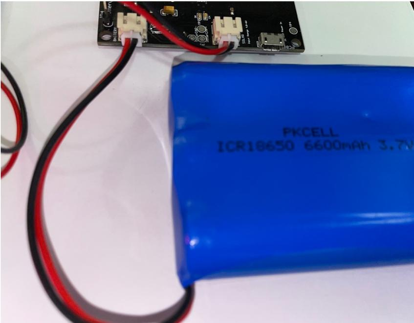
**Step 10:** Push the switch on the SunAirPlus2 (Part F) board away from the battery connector. You should see LED lights come on on both boards and see the white Interrupt LED light up (and then go off shortly) on the ThunderBoard. If the white LED on the ThunderBoard (Part D) does not go out, you have plugged your 50cm Grove cable into the wrong plug on the ThunderBoard (Part D) or on the MiniProPlus (Part A). Go back to Step 3.
