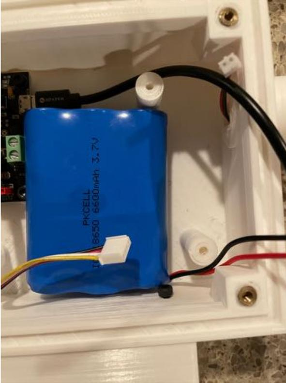
Step 8: Making sure the SunAirPlus2 switch is in the off position (slide towards the battery connector), plug in the battery (Part G) to the JST-2 connector marked Battery on the SunAirPlus2 Board (Part F) as shown below.
