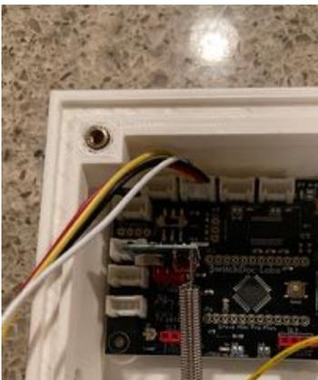
Step 5: Plug the 20cm Grove cable (Part H) into the J7-I2C Grove connector on the MiniProPlus (Part A).
