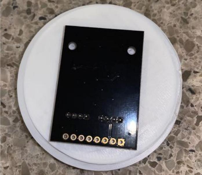
Step 18: Screw the Saucer Lightning Top (Part P) onto the Saucer Lightning Base (Part Q). This forms the Lightning Saucer Assembly.
