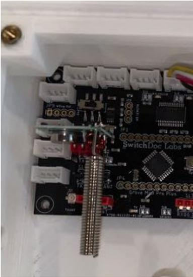
Step 4: Take the 50cm Grove Cable (Part H) and plug it into the Grove connector marked J5-I2C on the MiniProPlus board (Part A). Route it out the hole in the bottom box (Part I).
