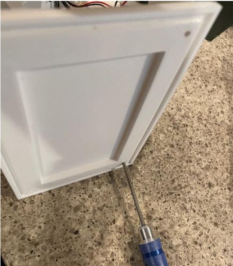
Step 3: Take the 510mm Screen Spline and push it into the Box Top (Part J) channel. Start in the middle of a long side. This becomes the bottom of the Box Top (Part J).
