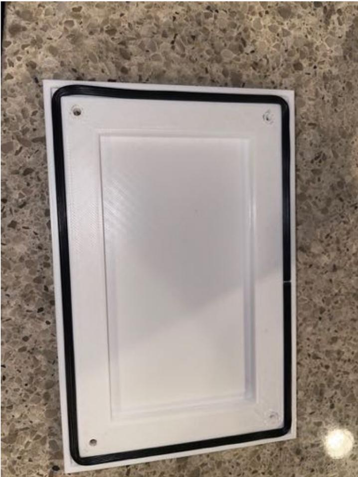
Step 4: Screw down the Box Top (Part J) with the spline gap at the bottom. Start all four 8mm screws until they just start into the brass inserts on the bottom box (Part I) and then go around and tighten all the screws down (but not too tightly!). This process adjusts for any minor alignment issues with your 3D Printer.
