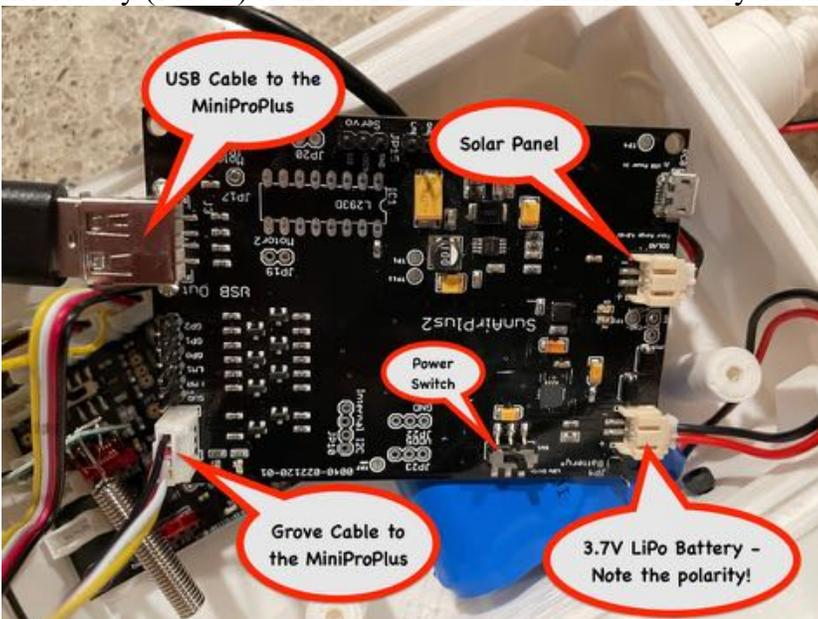
Step 9: Attach the Solar Panel (Part E) JST-2 plug to the JST-2 connector on the SunAirPlus2 (F) board as shown above.
