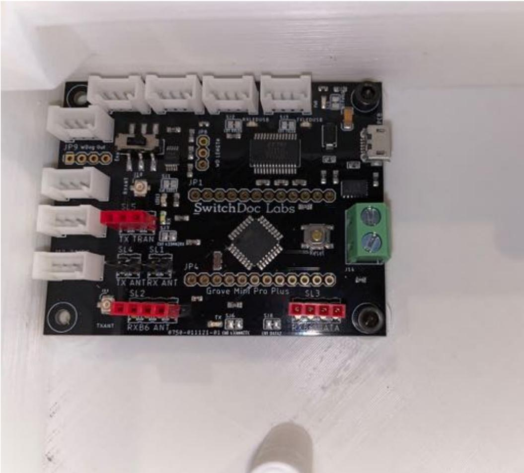
Step 3: Take the 433MHz transmitter (Part C) and plug it into the TX header on the MiniProPlus board (Part A). Make sure you have bent the pins slightly (down-up-down) to ensure that you get a good connection.
