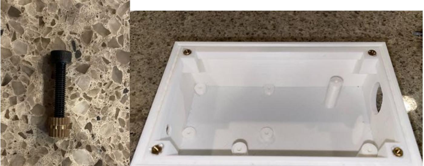
Step 2: Attach the MiniProPlus (Part A) to the bottom box (Part I) using two 5mm screws as shown below. As always, tighten, but don't over tighten the screws as you will strip the plastic threads.
