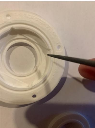
Step 18: Place the smaller O-Ring in the SkyCam Window Top (Part L). It does not need to fit perfectly, but put as much of it the ring slot as possible.
