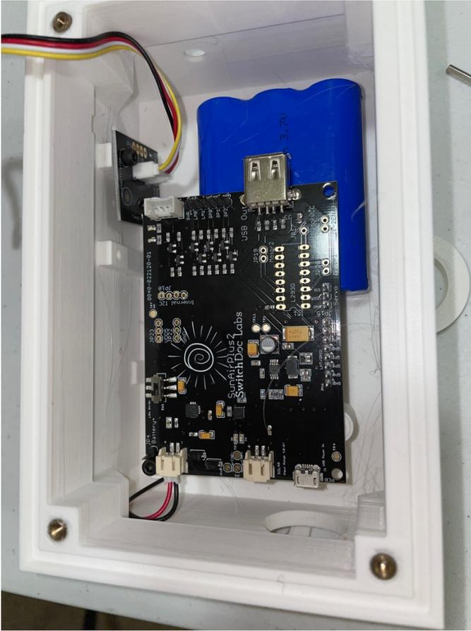
Step 10: Plug the remaining 20cm Grove cable (Part C) into the I2C Grove connector on the SunAirPlus (Part B) board.
