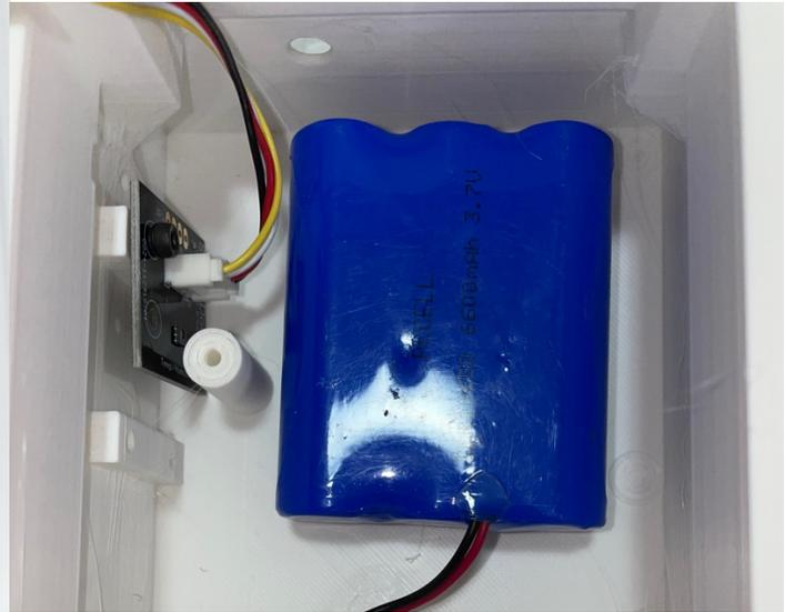
Step 9: Plug your LiPo battery into the battery JS2 plug (across from the switch in the lower right corner). Take your SunAirPlus Board (Part B), make sure the switch is off, and screw it down using two 5mm screws. Take care not to break the pylons or tight so much to strip the threads. You will only use the two mounting holes on the left side of the board.
