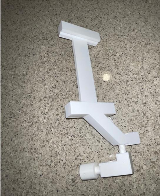
Step 22: Slide the Solar Panel (Part D) into the slots on the Solar Bracket (Part O) with the wires facing down. If it is too loose, secure with tape or glue. Your Solar Bracket Assembly is complete. If your wires are too short given your chosen position, you can solder a longer pair of wires to the panel, or you can buy a JST-2 Extender from SwitchDoc Labs ( <https://shop.switchdoc.com/products/jst-ph-battery-extension-cable-500mm> ).
