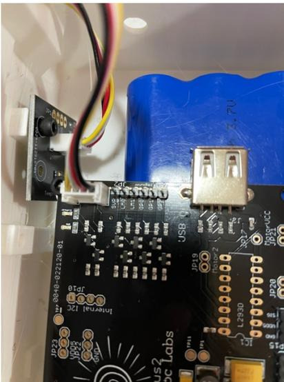
Step 11: Plug the Type A end of the USB micro to USB Type A cable (Part F) into the SunAirPlus Board (Part B). If the USB Plug won't fit, the remove the SunAirPlus board (Part B), attach the USB Cable (Part F) and replace the SunAirPlus Board (Part B).
