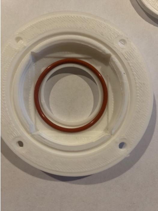
Step 19: Now gently push the quartz window into the SkyCam Window Top (Part L). Make sure it is resting on top of the O-ring.
