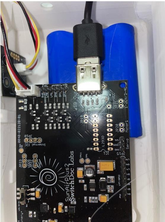
Step 12: Attach the Solar Panel (Part D) JST-2 plug to the JST-2 connector on the SunAirPlus (Part B) board as shown above. Remove the plastic covering of the Solar Panel at this time.
