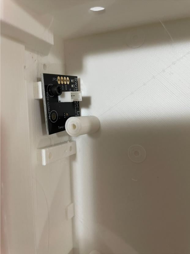
Step 6: Take a 20cm Grove Cable (Part C) and plug it into the Grove connector on the HDC1080 Temperature and Humidity Sensor (Part E).
