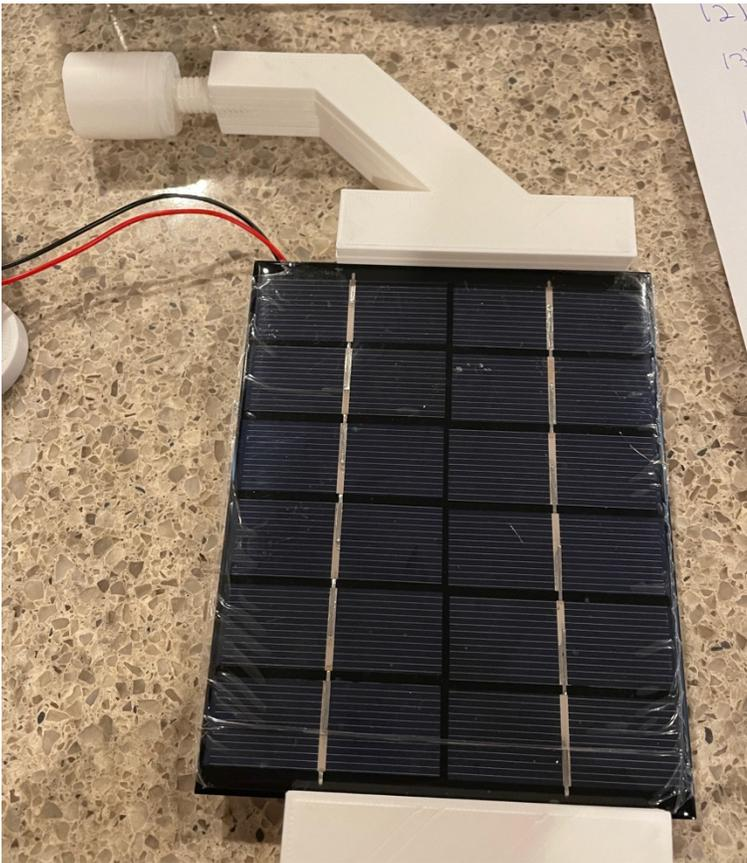
Step 23: Slide the complete Solar Bracket Assembly into the Main SkyCam Box (Part J) hole on the right side, making sure all wires are in the slot and not being pinched by the assembly. Align the holes on both sides of the Slotted Box Plug (Part P) with the lock screws. Tighten the lock screws, again not too tightly or you will strip the 3D printed threads inside the Slotted Box Plug (Part P).
