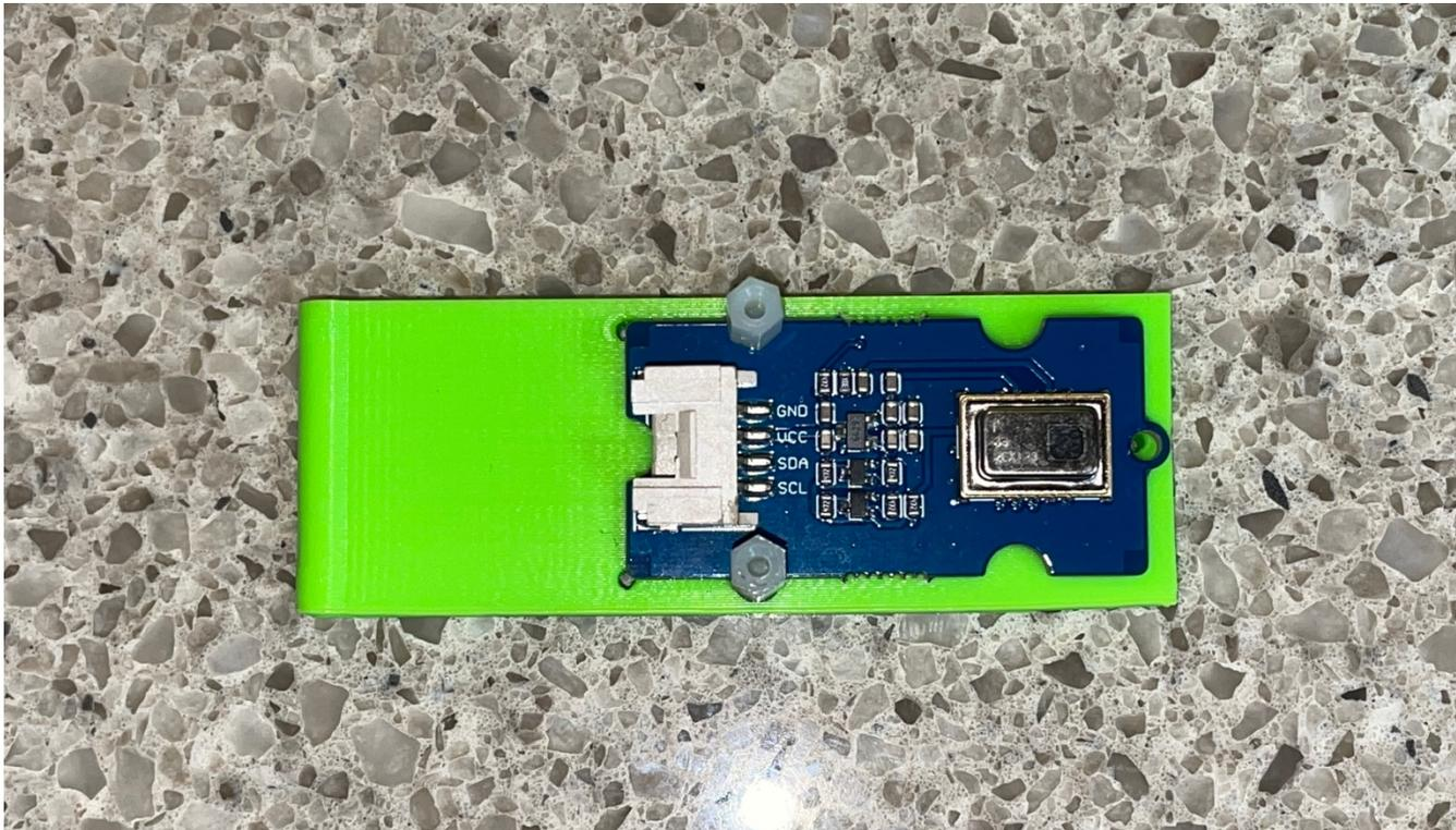
Step 8) Slide the Mount into the Mount Base (Part K) and screw it to the Hydroponics Light Holder (Part A) as shown. If the AMG8833 Mount is not tight, use a M3 set screw to hold it in position by threading it into the hole on the Mount Base.
