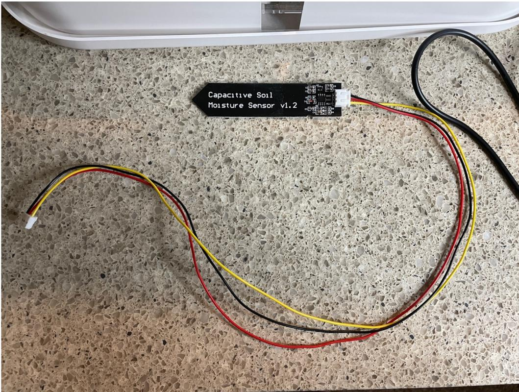
Step 20) Plug the other end of the cable from the Capacitive sensor (Part F) into the SmartGarden3 Wireless Extender port marked "MS4" on the Extender Board. Route it through the leftmost hole on the back of the Wireless Extender.
