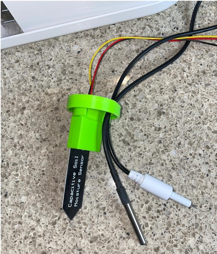
Step 22) Push the assembled 3D Printed Hydroponics Sensor Mount (Part M) into the rightmost hole of the Hydroponics Unit (Part A) as shown.
