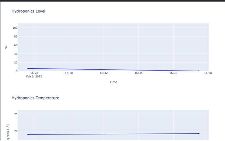
If you don't see information from your temperature sensor or aren't seeing a very low water level, go back and check your wiring. It is normal that the TDS sensor reads 0.0ppm with no water in the unit.
