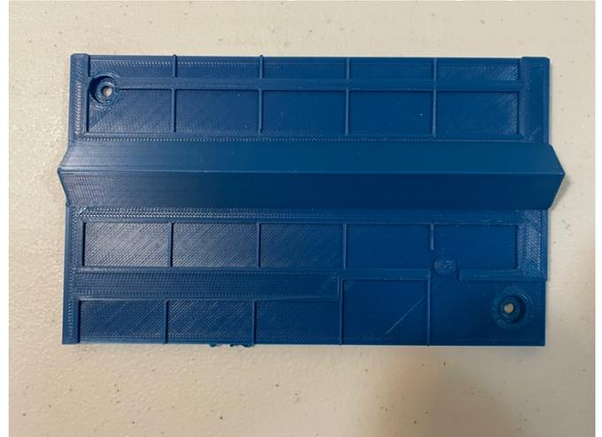
Part M – 3D Printed Hydroponics Sensor Mount
