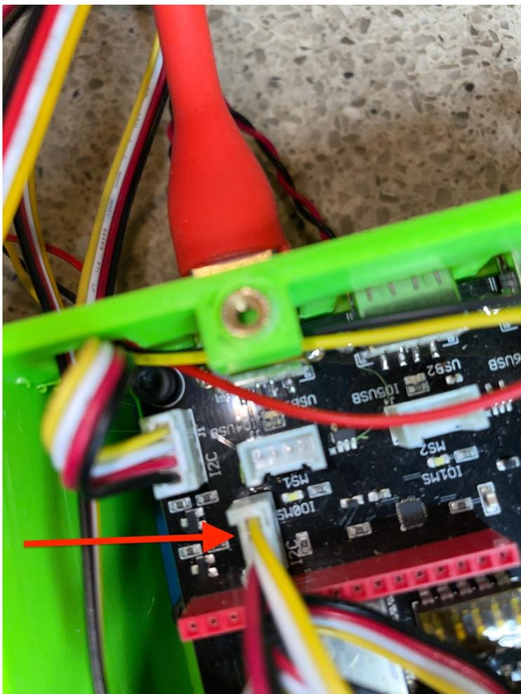
Step 26) Take the other end of the 50cm Grove Cable (Part G) from Step 25 and plug it into the Wire Hub Board (Part B) in the bottom slot marked I2C (shown below).
