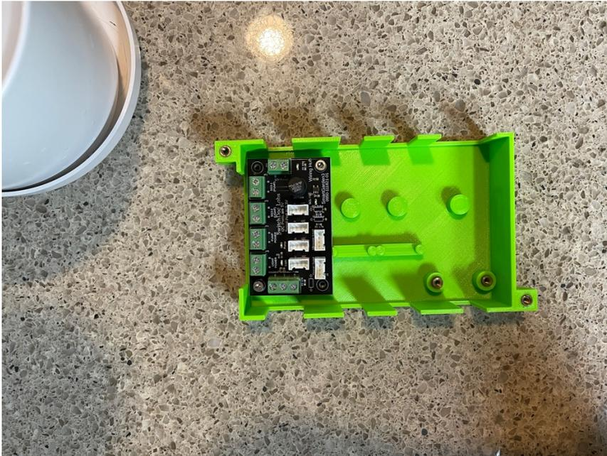
Step 6) Install the Grove TDS Board (Part E) into the 3D Printed Hydroponics Wire Hub Base (Part J) as shown. If it doesn't snap fit, then use a small amount of glue on the back to hold it on the upper post.
